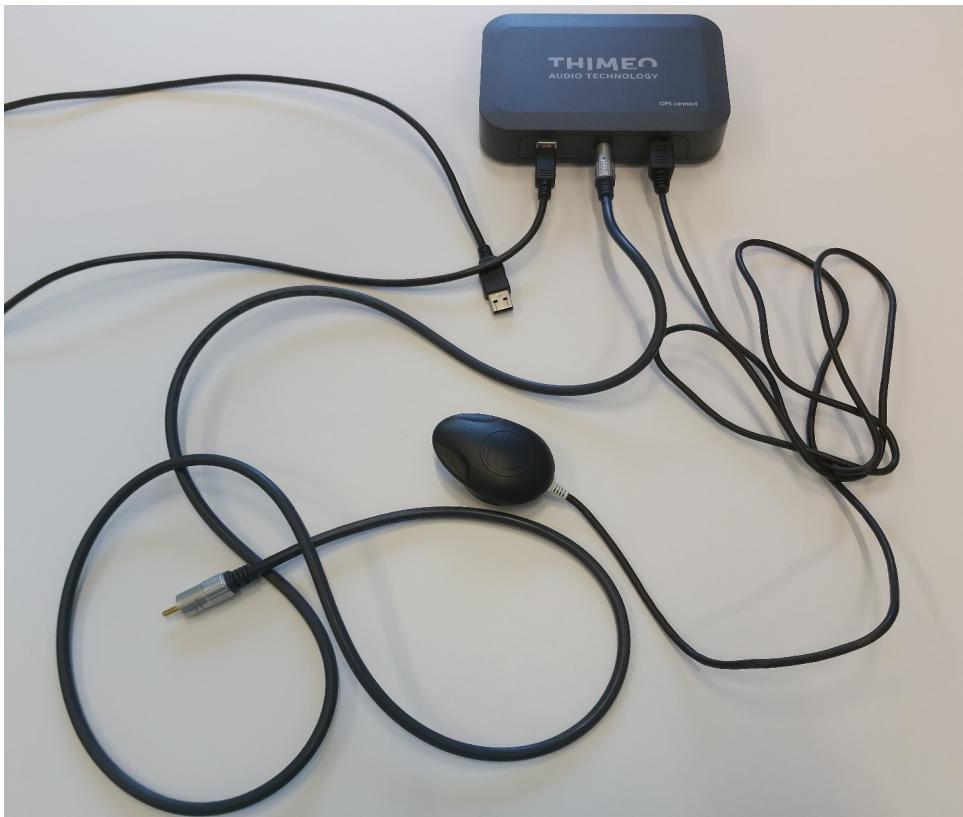
Connect the GPS receiver to the Thimeo Connect box, and connect a USB cable from the Thimeo Connect box to your computer. Then connect an audio cable from the Thimeo Connect box into the *left channel* sound card input that is coupled to the output that will be used for the MPX signal. If you're using Windows, use a sound card that supports ASIO, and select an ASIO sound card in the sound card dropdown list. Synchronization will not work without ASIO on Windows.
