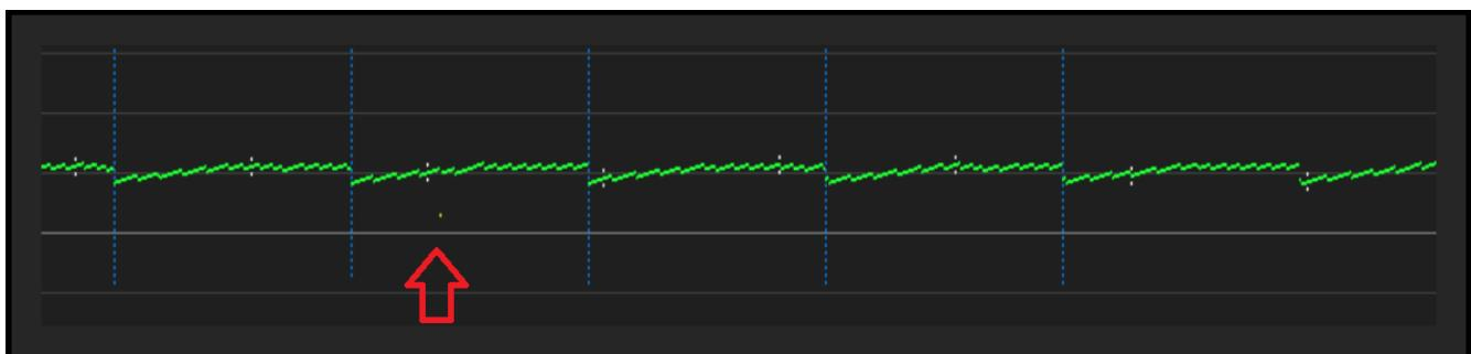
If you see occurrences like this, you can see that the yellow packet was recovered only just in time, and that could be a reason to increase the Delay a bit. Or reduce the forward error correction span setting.
