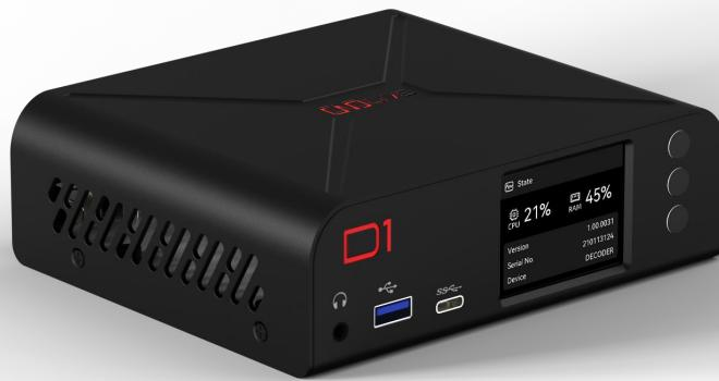
CNDLive D1 is an advanced and professional video decoder. It comes with HDMI 2.0 and 3G-SDI dual outputs, capable of dealing with multiple video formats and coding standard.
