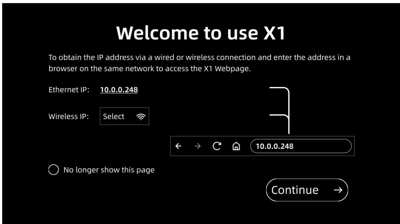
For example, "10.0.0.248" indicates that the device has successfully acquired an IP address through the wired network.
