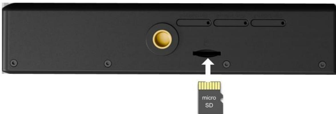
Make sure that your TF/SD card is inserted into the TF card slot of the device in the correct orientation as shown in the diagram.
